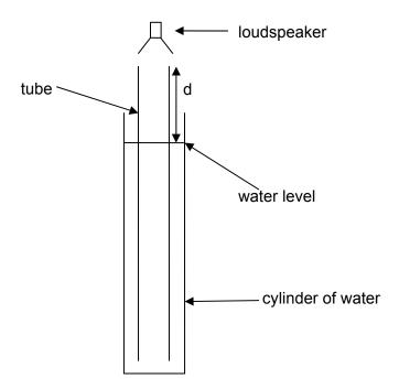
The first resonance is heard when the length of the air column above the water (labelled **d** in the diagram) is 17.0 cm and a second is heard when the length of the air column is 49.0 cm.
